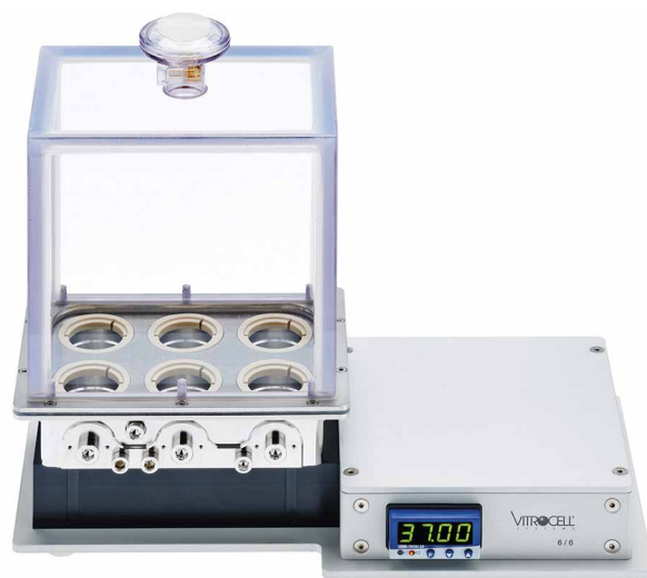
Device for in vitro exposure of lung cells to aerosolised nanomaterials under physiologically realistic conditions (VITROCELL CLOUD 6).
